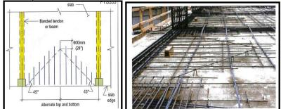
(iv) the provision of minimum longitudinal steel (untensioned reinforcement) at column positions for all flat slabs of at least 0.075% of the gross concrete cross-sectional area, concentrated between lines that are 1.5 times the slab depth either side of the width of the column and extending 0.2L into the span, L [cl.6.10.6 TR.43]
